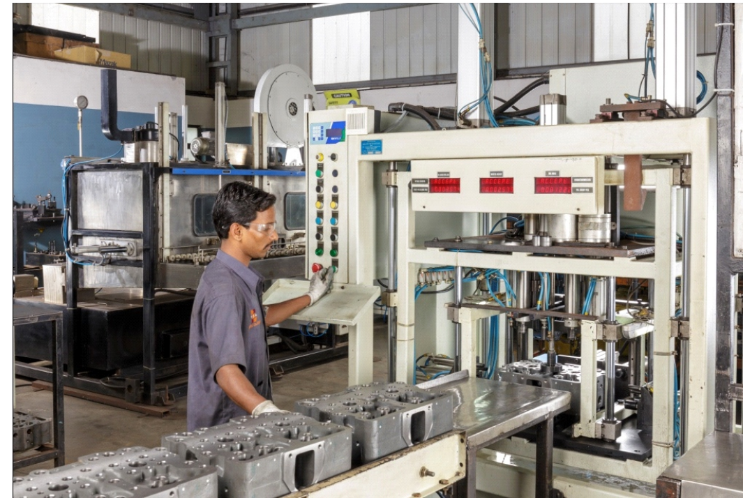
Leak Testing Machine Accuracy :- 0.0009 bar.
